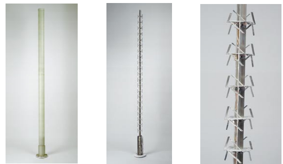
21 Elements, 11 Elements Excited 11-Way Power Divider at Base Equal-Line-Length Cables to Elements
